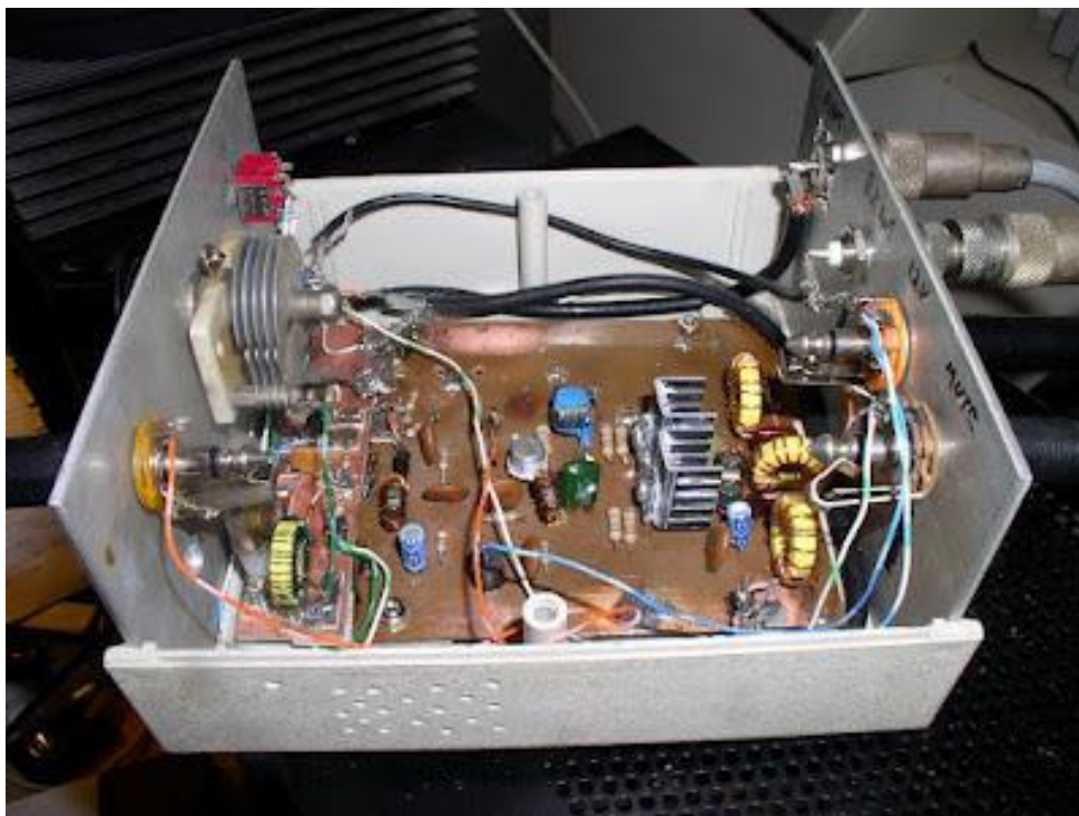
March 2013 Rebuild of the VXO 6 watt
