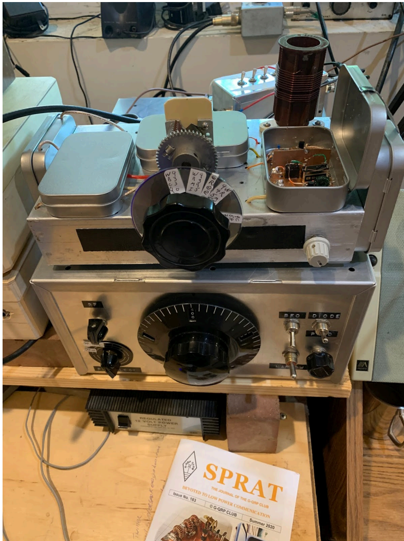
Q-31 with the can for the ceramic filters open
