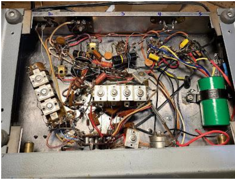
Recapping in process. Hayseed electrolytic in green can.. Old tubular caps being replaced by new yellow caps.
