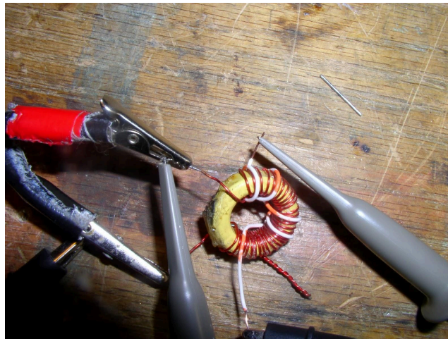
Opposite "sense" winding and resulting phase shift
