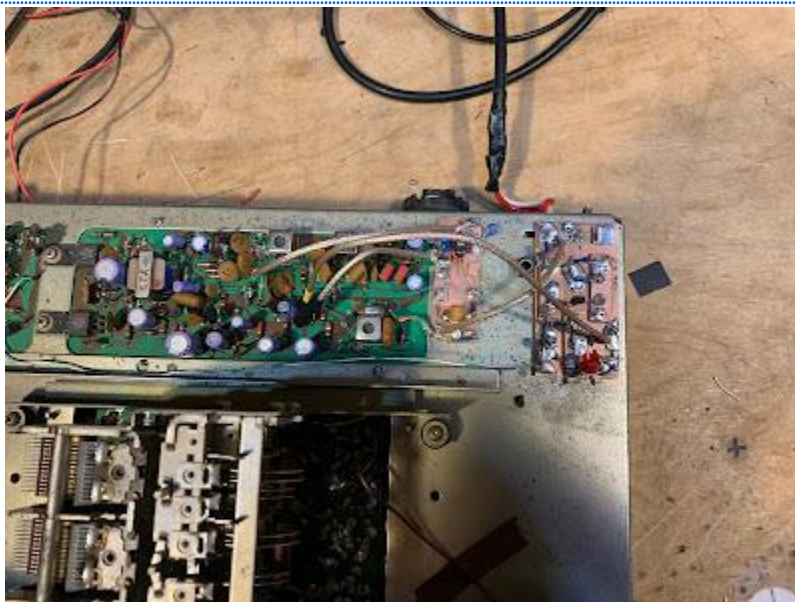
Diode product detector on the left, BFO amp in the right
