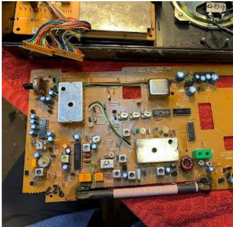
DX-390 Main Board. Note kludged toroidal replacment for L10 (just above ferrite antenna)
