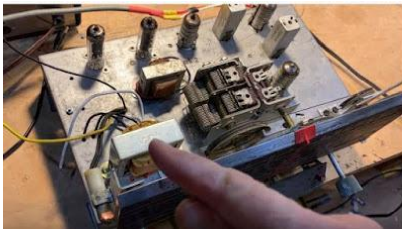
Where I placed the isolation transformer on both my S-38Es
