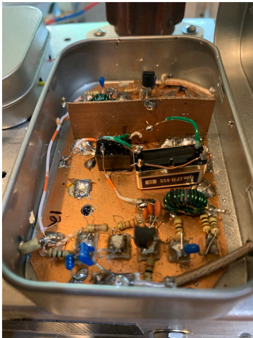
\pm 6 kc filter upper left, 455B wide filter to the lower right.
